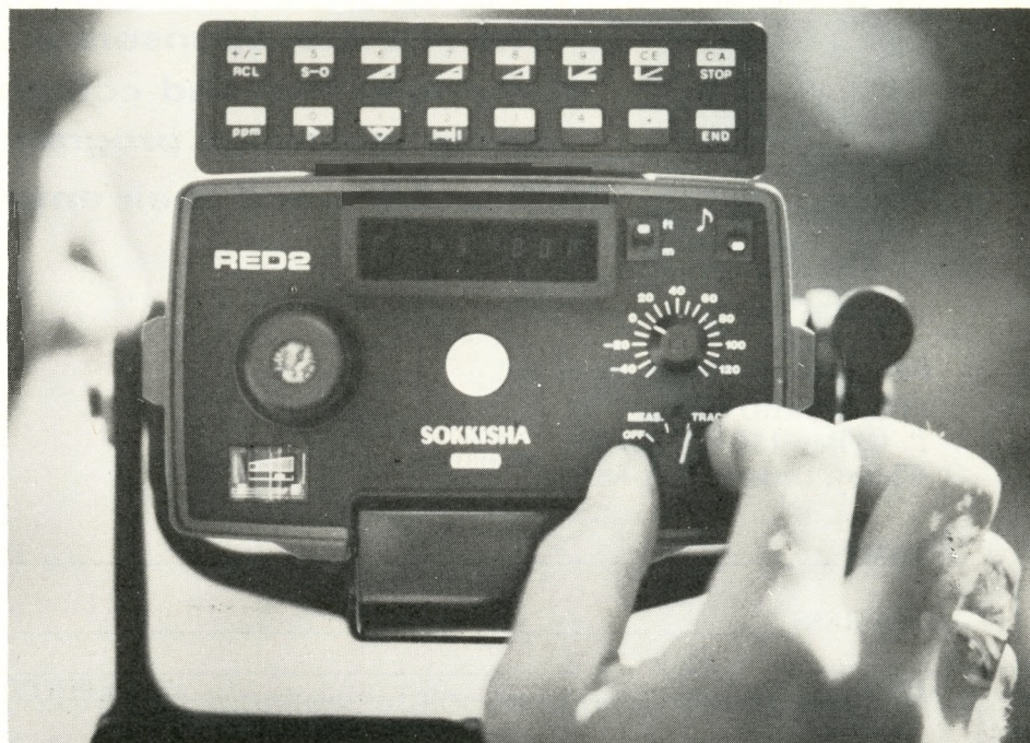
Above is an electronic distance measuring device which is mounted on the theodolite.
